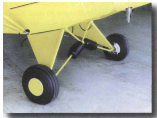
Figure 2-14. Spring steel (left) and bungee cord struts (right) accept and transmit shocks to the airplane at an acceptable rate.
