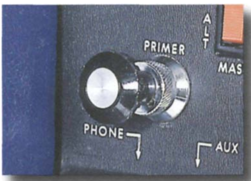
Figure 2-35. This manual pump-type primer can be used to help start a cold engine.
