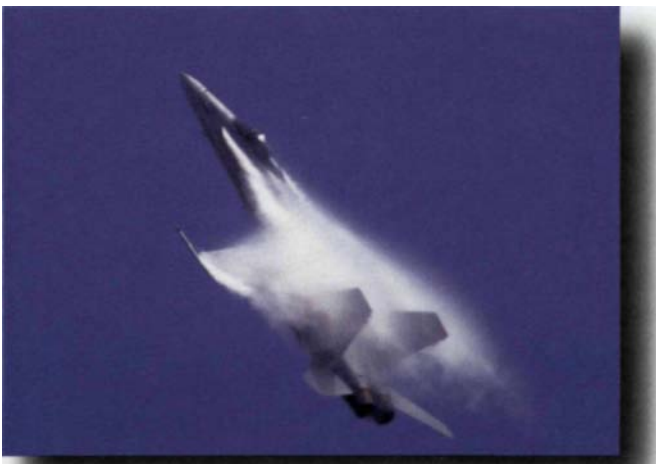
Figure 3-66. When a pilot pulls G's during aerobatic maneuvers in warm, humid conditions, the increased wing loading and decreased pressure above the wings can contribute to the formation of a distinctive condensation cloud.
