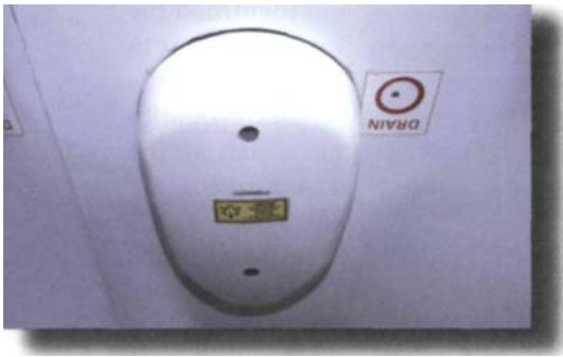
Figure 9-33. On this aircraft, the directional antenna and the sense antenna are combined in a single unit.
