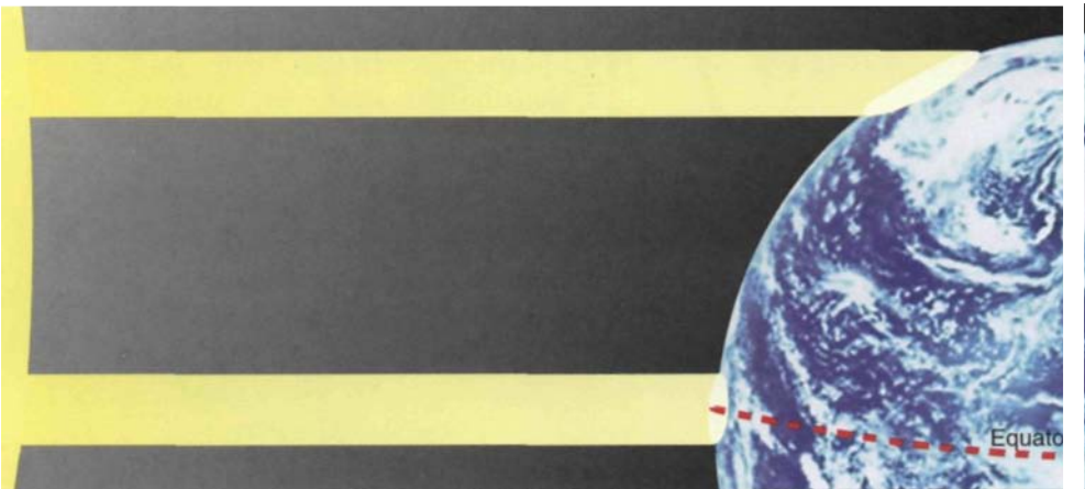
Figure 6-4. Although the same amounts of solar energy strike the earth at the equator and near the pole, the energy is spread over a much larger surface area near the pole than at the equator.
