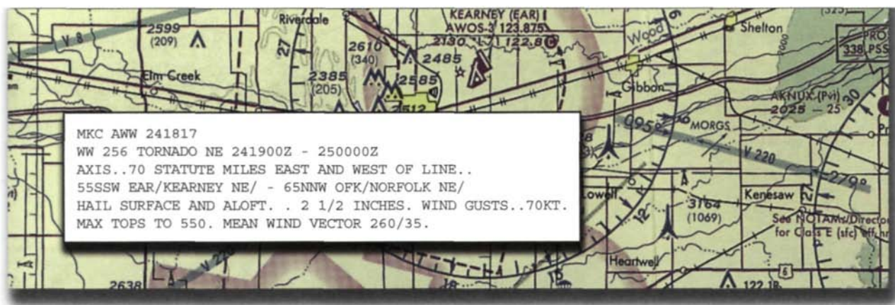
Figure 7-15. AWW in the header identifies this report as a severe weather forecast alert. This message warns of possible tornado activity in Nebraska and defines the watch area. Hail and high winds also are possible. A detailed severe weather watch bulletin (WW) immediately follows the alert message.
