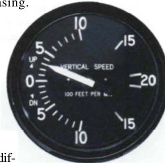
Figure 2-75. The vertical speed indicator tells you how fast you are climbing or descending. The VSI on the left shows a 300 f.p.m. descent, while the VSI on the right reflects a 300 f.p.m. climb.
