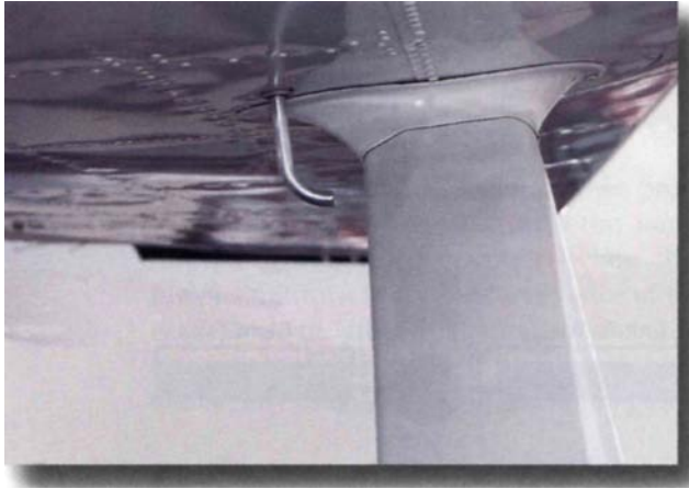
Figure 2-36. On this Cessna 172, the left tank is vented through a tube (shown) while the right tank is vented through the filler cap.
