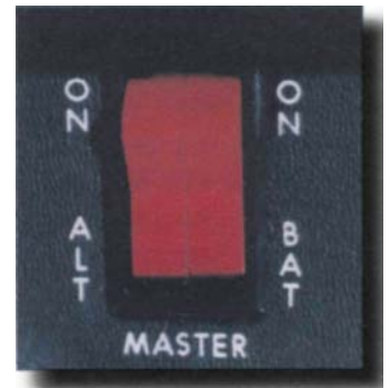
Figure 2-59. Most airplanes use a split-rocker type master switch. The right half is labeled BAT and controls all power to the electrical system. The left half is labeled ALT and controls the alternator.
