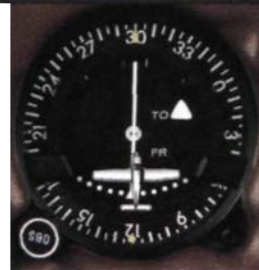
Figure 9-21. To determine your position relative to a VOR, it may help to visualize your airplane at the bottom of the VOR indicator.
