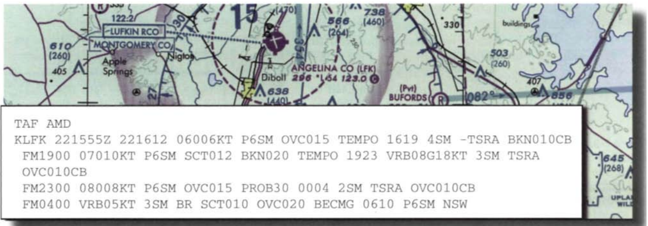
Figure 7-10. With a few exceptions, the codes used in the TAF are similar to those used in the METAR.
