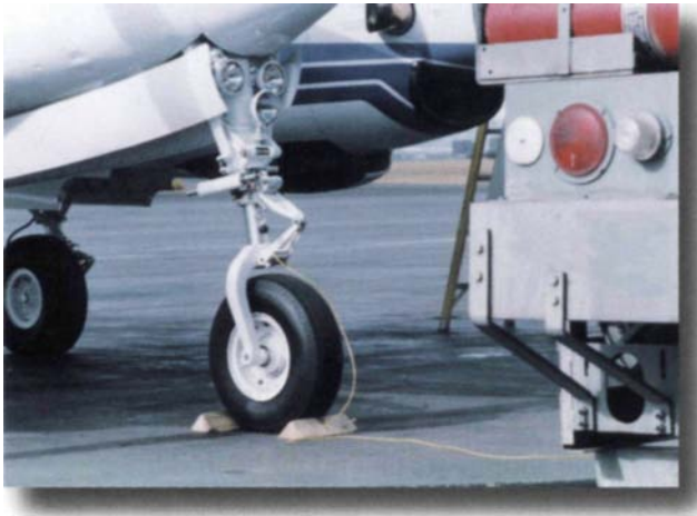
Figure 2-41. A ground wire should be attached to the airplane during all refueling operations.
