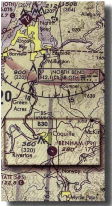
Figure 9-28. In this example, your VOR indicator should display 164^\circ (\pm 6^\circ) FROM the North Bend VORTAC as you overfly the east edge of the town of Coquille.
