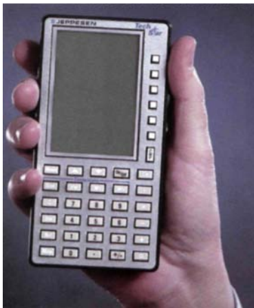
Figure 8-60. The keyboard of the TechStar flight computer is shown here. Study the manual to familiarize yourself with the locations and functions of the various keys.
