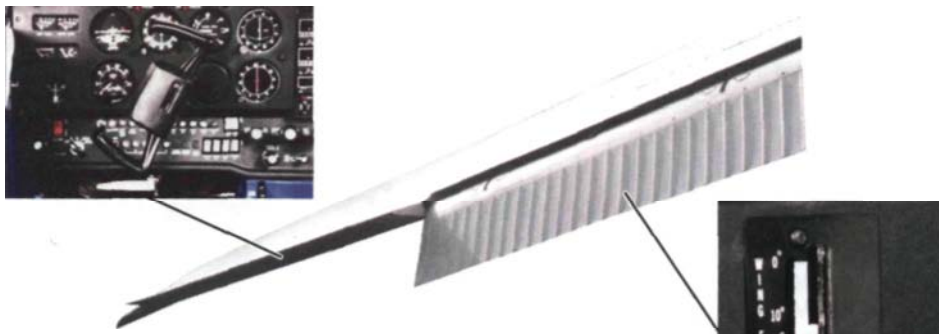
Figure 2-5. The ailerons are normally connected to the control wheel by a series of chains, cables, bellcranks, and pulleys. When you turn the wheel to the left, the left aileron moves up and the right moves down. During flight, this is how you start a turn to the left. Turning the wheel to the right has the opposite effect. You can operate the flaps using a switch or handle located in the cockpit. They are used primarily for takeoffs and landings.
