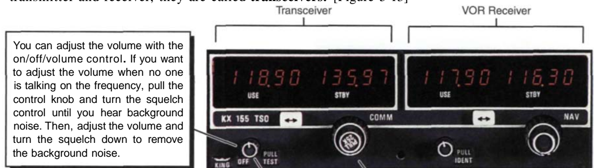
Figure 5-13. Most VHF radios have both communication and VOR navigation receiver capability in one unit. Use of the VOR receiver for navigation is discussed in Chapter 9.
