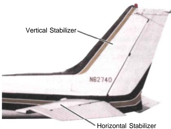
Figure 2-6. The vertical and horizontal stabilizers are located on the empennage.
