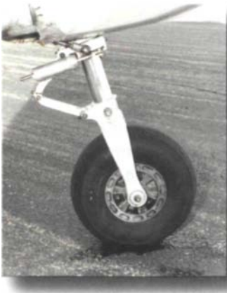
Figure 2-15. The oleo strut consists of an enclosed cylinder which houses a piston, oil, and air. It absorbs pressure rapidly and then slowly releases it.
