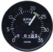
Figure 2-54. The propeller control changes the pitch of the propeller blades, thus controlling engine r.p.m., which is indicated on the tachometer.
