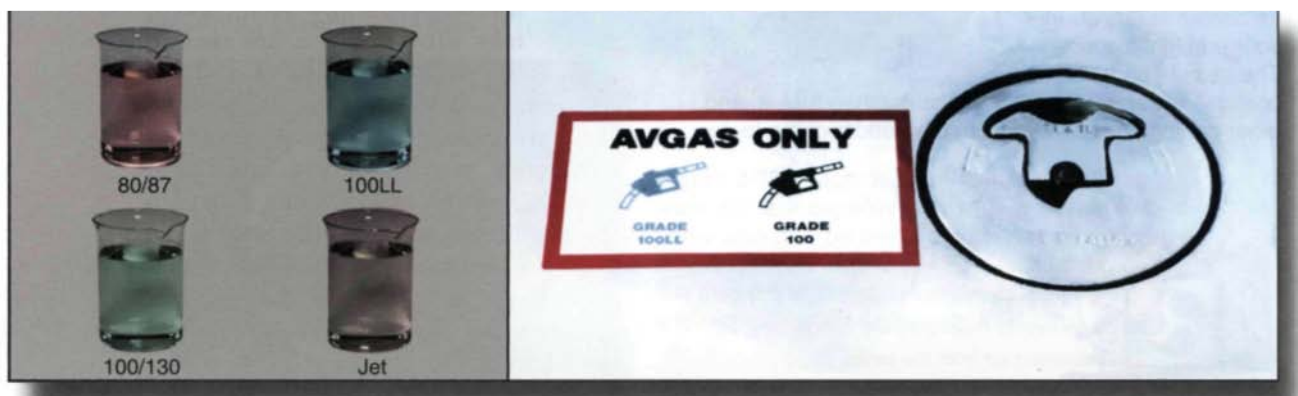
Figure 2-42. Color coding of fuel and placement of decals near fuel tank filler caps helps ensure that you use the proper grade of fuel.
