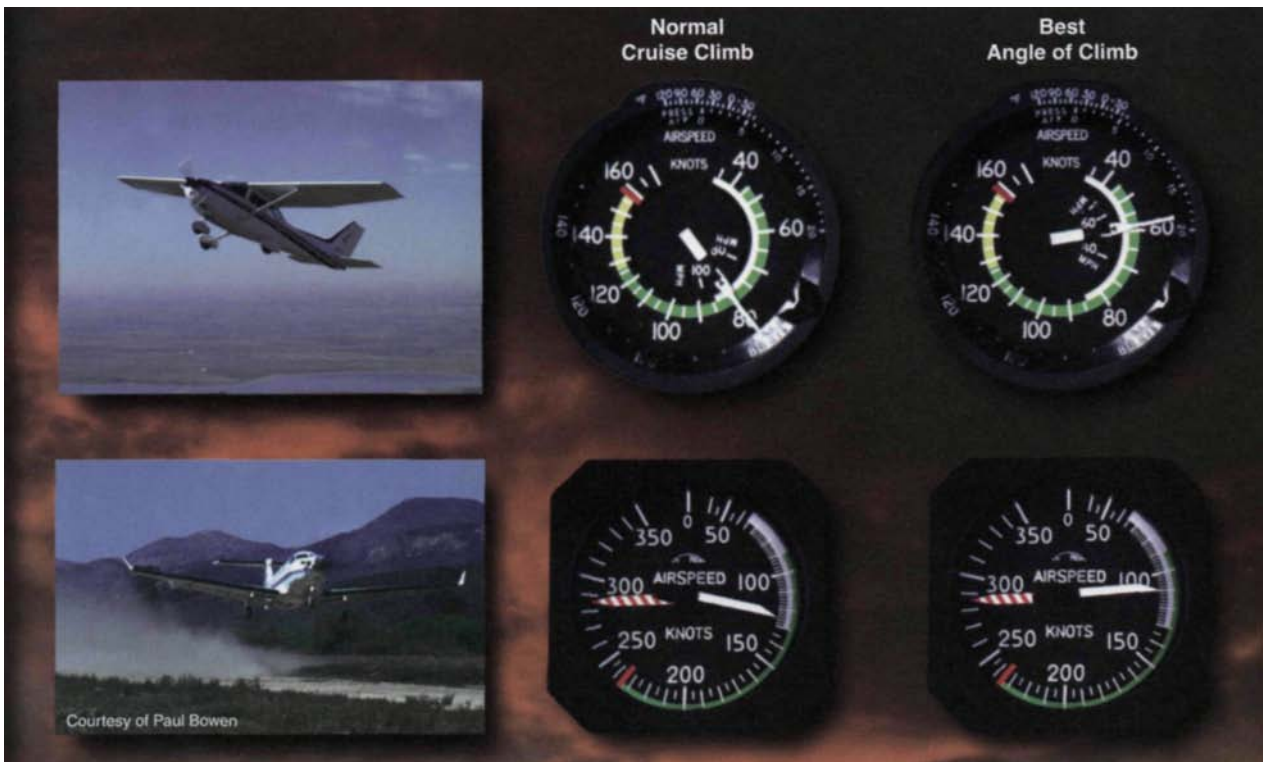
Figure 8-12. Climb airspeeds vary between aircraft. For example, the Cessna 172 has a normal cruise climb speed of 75-85 knots, however the pilot's operating handbook recommends 59 knots for the best angle-of-climb airspeed. The high-performance Pilatus PC-12 has a normal cruise climb airspeed of 125 knots and a best angle-of-climb speed of 110 knots.
