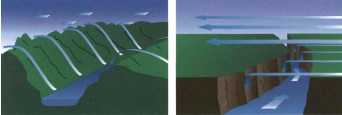
Figure 6-47. Winds moving across a gentle sloping valley (left) produce winds which generally follow the valley contour. In a very narrow canyon with strong crosswinds (right), conditions may be significantly different. In this case, turbulence or downward motions occur on the downwind side of the valley. Additionally, airflow at the bottom of a narrow canyon can be turbulent due to sharp bends and limited space.
