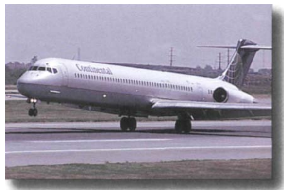
Figure 2-12. Tricycle landing gear is used on many of today's aircraft, including almost all modern transport category airplanes.
