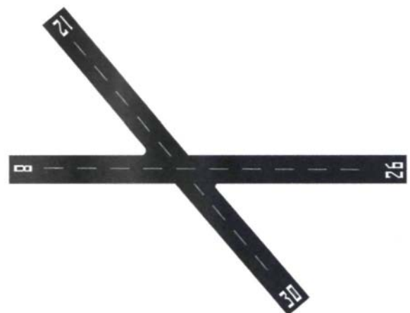
Figure 4-14. When possible, you should select the runway that is the closest to paralleling the direction of the wind. In this case, Runway 8 would be the logical choice for takeoff and landing into the wind.
