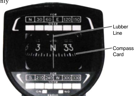
Figure 2-88. The compass doesn't work on gyroscopic principles, but you will use it frequently to help correct for gyroscopic precession in the heading indicator.
