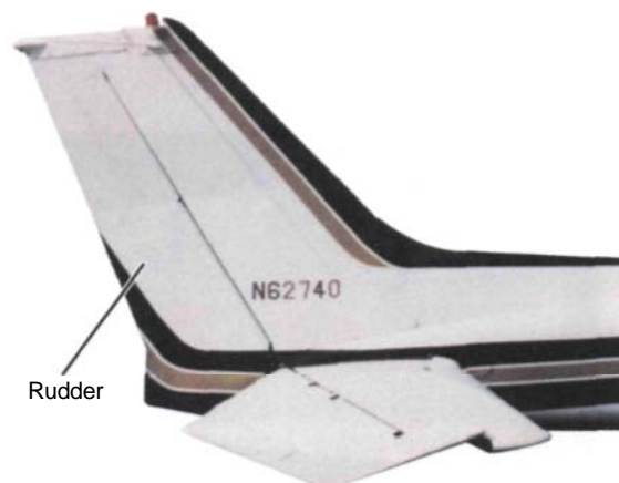
Figure 2-7. You operate the rudder with your feet, using pedals located in the cockpit. When you press the left rudder pedal, connecting cables move the rudder to the left which causes the airplane's nose to move to the left. Pressing the right pedal moves the rudder and nose to the right.
