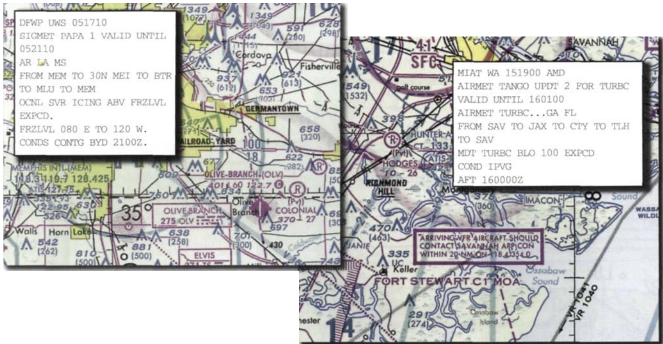
Figure 7-17. The first issuance of a SIGMET, as shown on the left, is labeled UWS (Urgent Weather SIGMET). PAPA 1 means it is the first issuance for a SIGMET phenomenon; PAPA 2 would be the second issuance for the same phenomenon. In the example on the right, AMD means this is an amended AIRMET of the phenomenon (moderate turbulence) identified as TANGO. The alphanumeric designator stays with the phenomenon even when it moves across the country.
