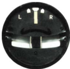
Figure 2-83. During your training, you may encounter either a turn-and-slip indicator or a turn coordinator; both provide essentially the same information.
