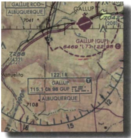
Figure 7-33. On a sectional chart, aT in the upper right corner of a navaid box indicates TWEB capability.
