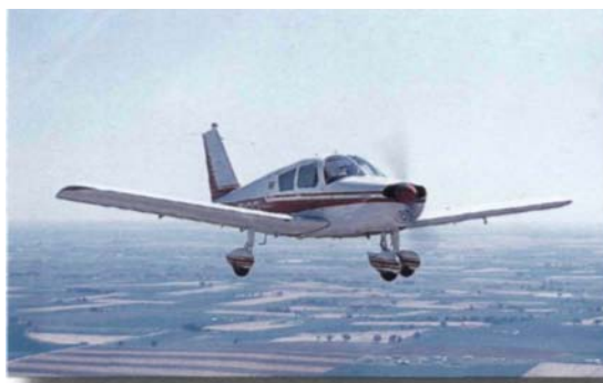
Figure 2-13. Most small training airplanes use fixed landing gear while higher performance airplanes are generally equipped with retractable landing gear.
