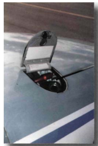
Figure 2-44. Engine oil level should be checked during your pre-flight inspection. Note the placard on the inside of the access panel.
