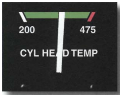
Figure 2-49. Like the other engine gauges, the normal range for the cylinder head temperature gauge is marked in green. You should compare the readings from the cylinder head temperature and oil temperature gauges. A disparity between the two may indicate a malfunction in one of the instruments. Oil and cylinder head temperatures above the normal operating range may indicate that you are using too much power with the mixture set too lean.
