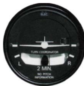
Figure 2-83. During your training, you may encounter either a turn-and-slip indicator or a turn coordinator; both provide essentially the same information.
