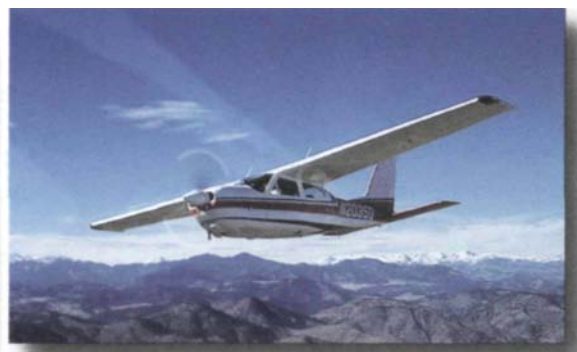
Figure 2-13. Most small training airplanes use fixed landing gear while higher performance airplanes are generally equipped with retractable landing gear.
