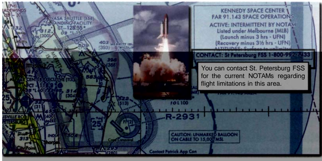
Figure 4-68. FAR 91.143 refers to flight limitations in the proximity of space flight operations.
