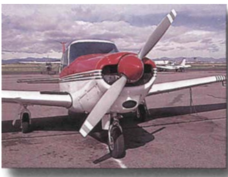
Figure 2-18. The propeller receives power from the engine and provides thrust to help move the airplane through the air.
