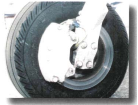
Figure 2-16. Most light general aviation airplanes use a hydraulically actuated disc brake on each main wheel.
