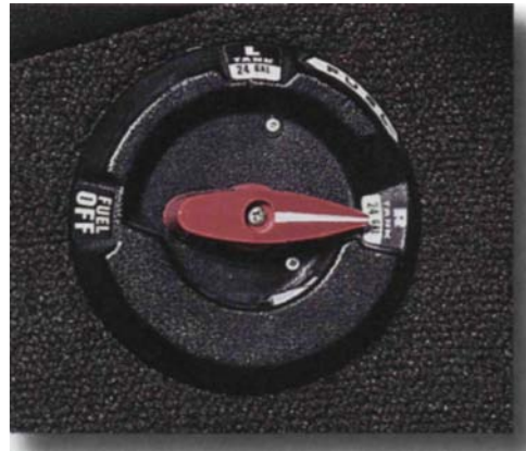
Figure 2-39. The three position fuel selector demands that you pay close attention to fuel tank quantities.
