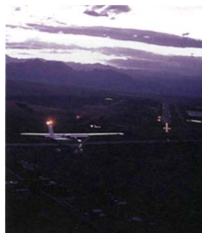
Figure 4-31. Approach light systems can aid you in locating the runway at night.
