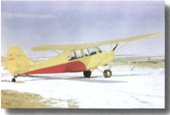
Figure 2-11. Because of the added clearance between the propeller and the ground, conventional gear airplanes are desirable for operations on unimproved fields.
