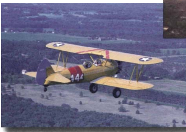
Figure 2-4. Monoplanes incorporate a single set of wings while biplanes use two sets of wings stacked vertically.
