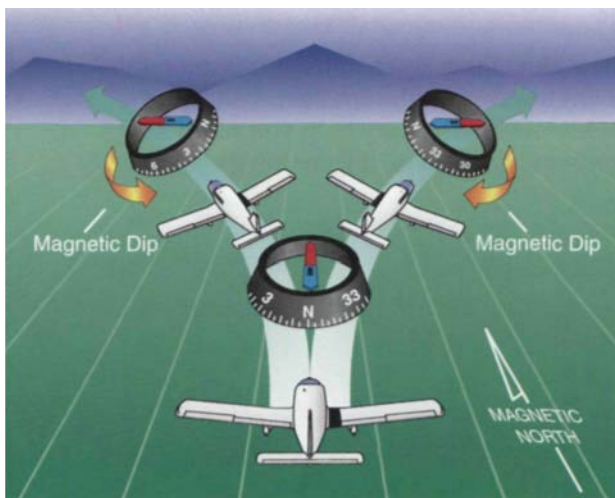
Figure 2-94. The left portion of the figure shows the initial tendency of the magnetic compass in a turn from a northerly heading. The initial turning error which occurs during turns from a southerly heading is shown on the right.
