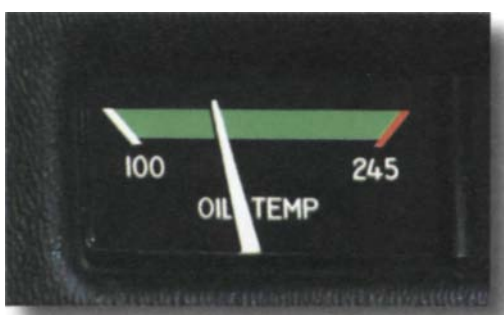
Figure 2-46. The oil temperature gauge measures the temperature of oil as it enters the engine. Normally, the green area shows the normal operating range and the red line indicates the maximum allowable temperature.
