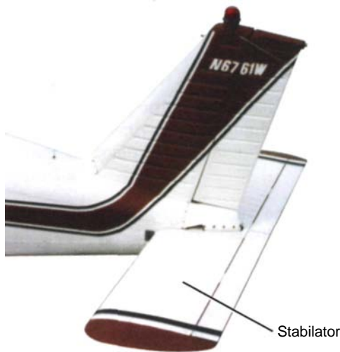
Figure 2-9. Some airplanes use a stabilator which performs the same function as the horizontal stabilizer/elevator combination.
