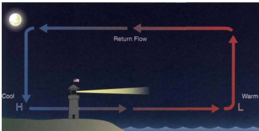
Figure 6-13. The land breeze, which flows offshore, is capped by a weaker onshore return flow. The land breeze can reach an altitude of 1,000 to 2,000 feet AGL and extend between 5 and 100 n.m. inland, depending on the conditions and the location.
