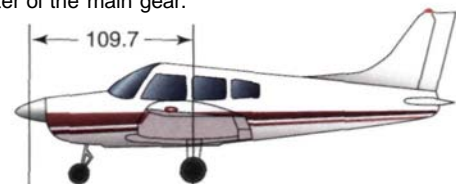
Figure 8-24. Although the datum is different in each of these airplanes, it is used in the same way for weight and balance calculations.
