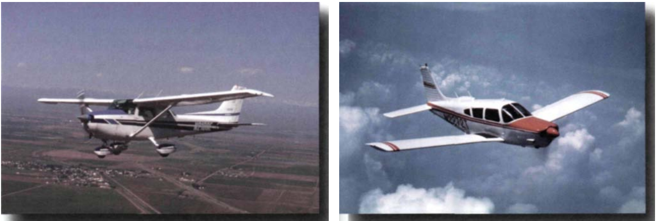
Figure 3-19. Design features such as wheel fairings and retractable landing gear can reduce both form and interference drag.
