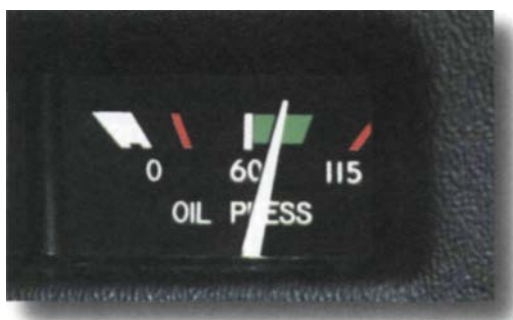
Figure 2-45. The oil pressure gauge measures the pressure in pounds per square inch (p.s.i.) of the oil supplied to the engine. Green typically indicates the normal operating range, while red indicates the minimum and maximum pressures.
