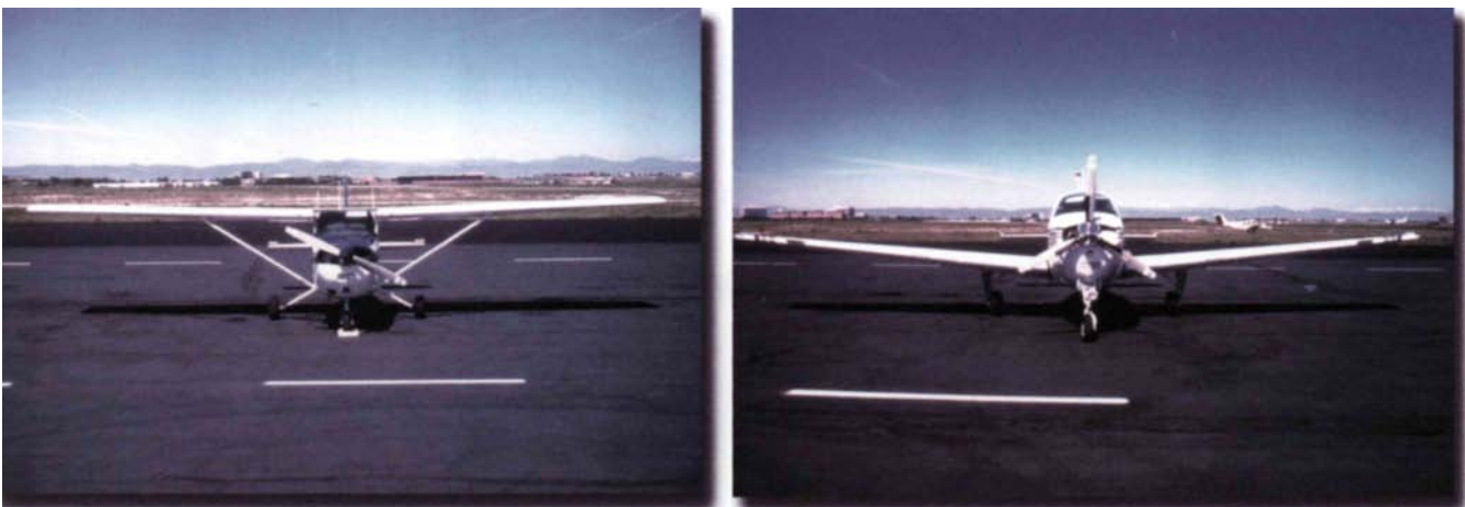
Figure 3-40. Since they are inherently more stable laterally, high-wing aircraft such as the Cessna 172 on the left are designed with less dihedral than the typical low-wing aircraft, as exhibited by the Beechcraft Bonanza on the right.
