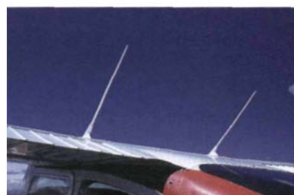
Figure 5-14. Normally, a VHF antenna is installed for each transceiver in the airplane. An airplane equipped with two transceivers usually has a microphone selector switch for the respective radios, so a second microphone is not required.
