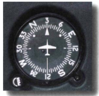
Figure 2-87. You should align the heading indicator (right) with the magnetic compass (left) before flight and check it at approximately 15-minute intervals during flight. When aligning the heading indicator while airborne, be certain you are in straight-and-level, unaccelerated flight, with the magnetic compass showing a steady indication.
