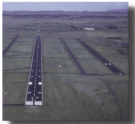
Figure 4-12. At large airports with heavy air traffic, it is common to have parallel runways. When assigning runways for takeoffs and landings, air traffic controllers will refer to these runways as "one-seven-left," and "one-seven-right."
