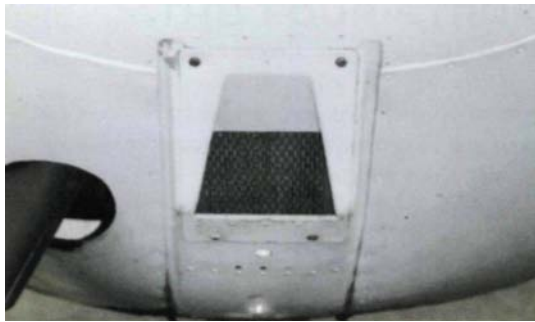
Figure 2-24. Engine intake air normally enters an intake port through an air filter.
