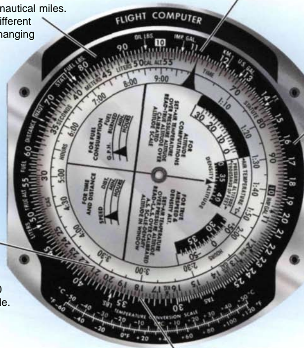
Figure 8-44. Suppose it has taken you 18 minutes to cover the distance between two landmarks that are 33.5 nautical miles apart, and you would like to know your ground-speed. Place the number of miles (33.5) over the number of minutes (18) and the speed index will point to the rate of speed in knots (112, in this example). Other calculations based on this speed can be made without changing the computer setting, for example, to find the number of minutes it will take to fly to your next checkpoint, just locate the distance on the A scale and read the time in minutes on the B scale.
