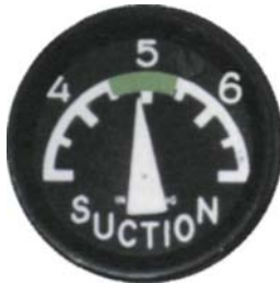
Figure 2-82. During flight, the suction gauge should indicate in the proper range. If not, your attitude and heading indicators may not be reliable.
