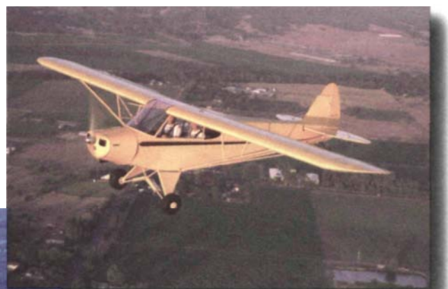
Figure 2-4. Monoplanes incorporate a single set of wings while biplanes use two sets of wings stacked vertically.
