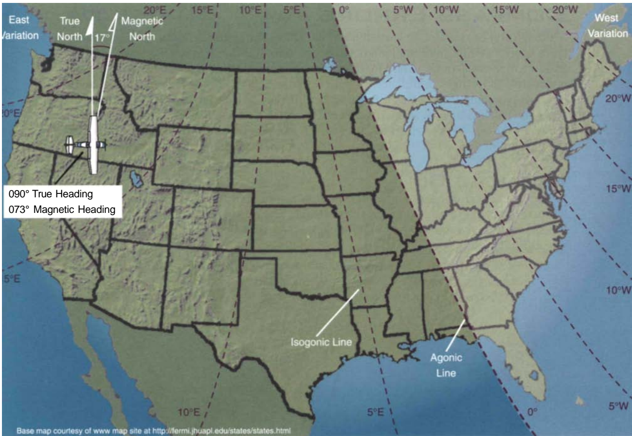
Figure 2-90. Variation at this point in the western United States is 17°. Since the magnetic north pole is located to the east of the true north pole in relation to this point, the variation is easterly. When the magnetic pole falls to the west of the true pole, variation is westerly. Isogonic lines connect points where the variation is equal, while the agonic line defines the points where the variation is zero.
